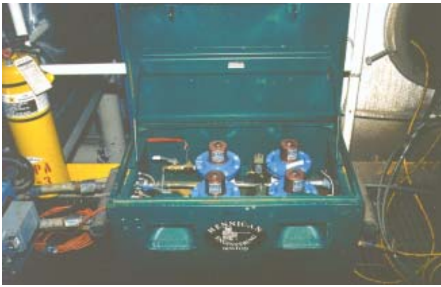
Hennigan Engineering's nitrogen gas pressure regulator provides full positive shut-off control, bypassing unused water from a work area at Indian Point Three nuclear power plant.
