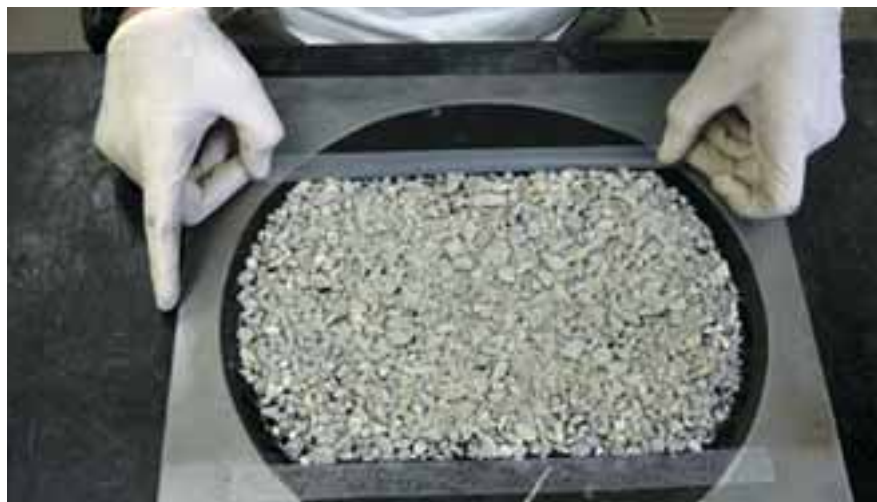
Top of page, right: Model Mobile Loading Simulator (MMLS3) accelerates wear on pavements; above, asphalt surface treatment aggregate test specimen is prepared at NCSU lab. Photo credits: North Carolina State University
