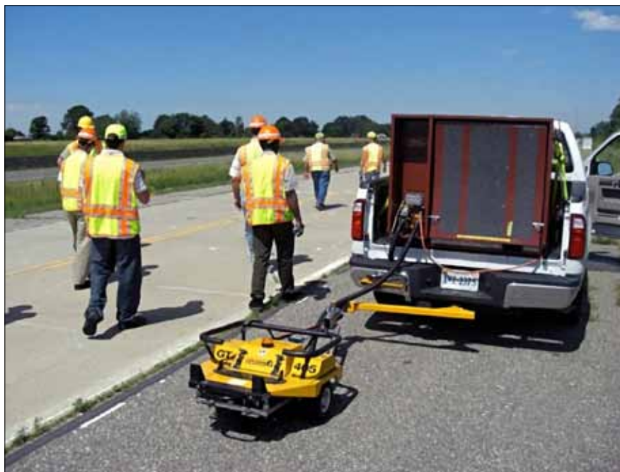
▲ In Virginia, a Findlay Irvine grip tester is used to measure continuous skid resistance measurements along the left wheel path of the travel lane of the test sections.
