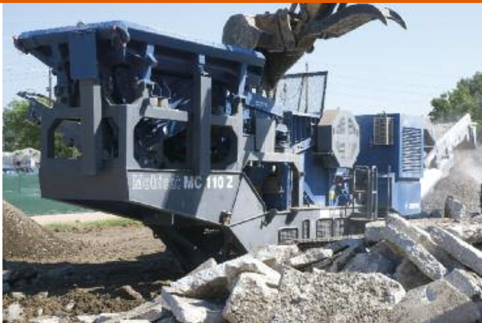
MC 110 Z quietly reduces concrete slabs with imbedded steel to a clean 2-in.-minus size
