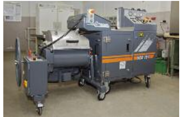
New WLM 30 mixer, left, adjacent to new WLB 10 S mobile lab
