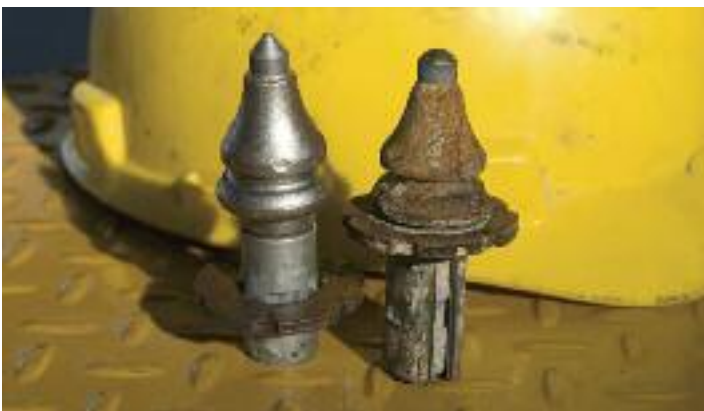
Fresh Rhino W1-10/S-R bit, left, compared to same bit after 36 miles of cutting; unique new design enhances productivity, longevity of bit life
