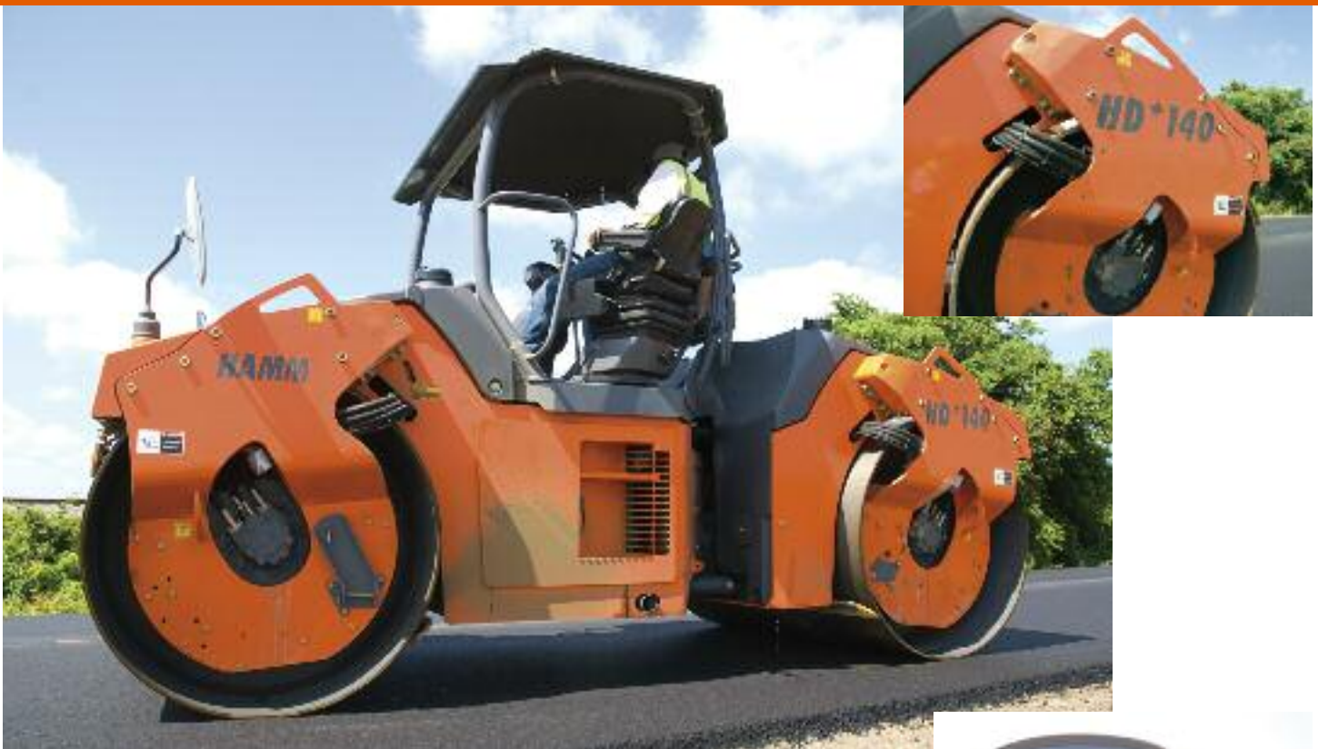
HD+ 140 VV is an articulated tandem roller, with operating weight of 14.5 tons and drum width of 84 in.
