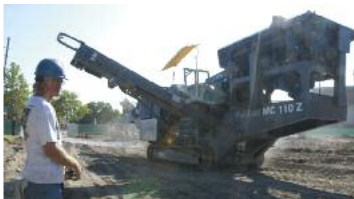
Operator uses remote control unit to 'walk' MC 110 Z to adjacent stockpile, but also to control crusher from cab of excavator/grapple
