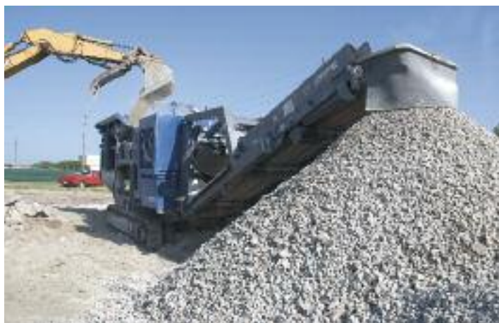
MC 110 Z is a track-mounted jaw crusher ideally suited for contractor work
