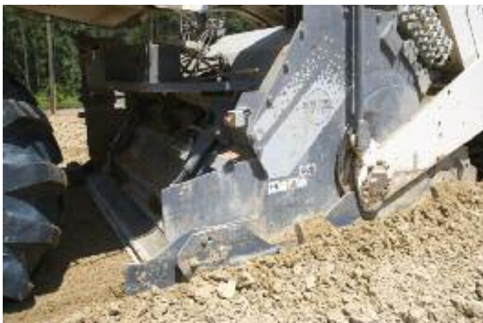
Gilchrist's WR 2400s can cut up to 20 in. deep at a 95-in. cutting width
