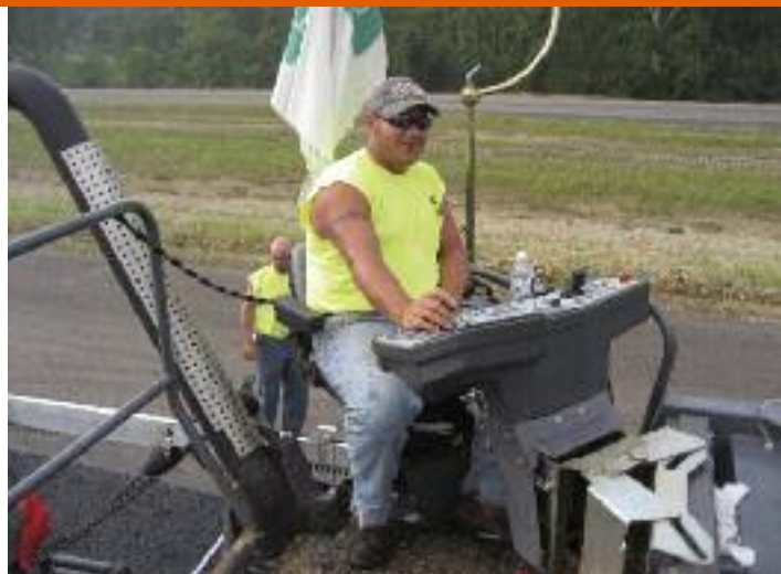
Enhanced visibility for operator above hopper and to side with swing-out seat improves chances of a successful placement
